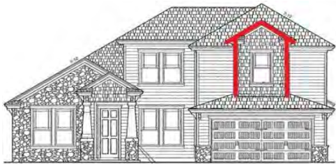
This home is unbalanced with too much weight over the garage, along with a rocket ship – not allowed.
